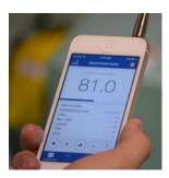
Need a quick sound check on the go? Turn your iOS device into a sound level meter by downloading a free app developed by researchers at the National Institute for Occupational Safety and Health (NIOSH). While the app is not meant to replace a professional sound level meter or noise dosimeter for compliance purposes, it does allows you to estimate A-weighted and C-weighted sound levels, maximum and peak levels and Time-Weighted Average (TWA) and Dose.
