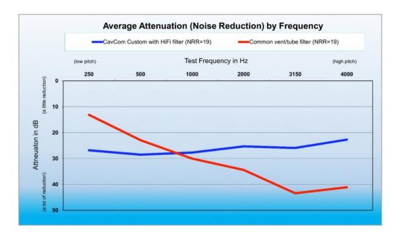
The older style tube filter (plotted in red) provides an uneven amount of protection very little reduction at low frequencies (pitches) and a great deal of reduction at high frequencies. This results in significant a "boomy" quality to sounds.
