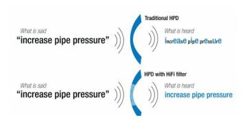
**Existing Hearing Loss.** For a worker with high frequency hearing impairment, a common occurrence, wearing hearing protectors can exacerbate the high frequency deficit. Speech intelligibility is reduced even further. A common complaint for people with hearing loss is "I can hear you talking, I just can't understand what you're saying." Overprotection can place a hearing-impaired worker, and those around him or her, at greater risk of miscommunications.
