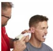
Each custom hearing protector [begins with an impression](#) of the individual's ears, which is used to digitally manufacture the earplug. Workers who were used to wearing "one-size-fits-most" hearing protection immediately felt the difference with *EarzON*®. Plus, for those required to utilize double hearing protection, the low-profile design was critical in ensuring both sets of protectors could be utilized without
